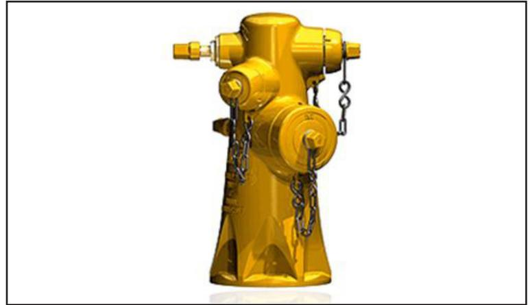
section. This top section is the main body where all the outlet valves and hardware are located. Each valve is associated to an independent outlet nozzle, which controls the flow of water. By attaching the hydrant wrench to the valve nut opposite the nozzle selected for use, and turning it counterclockwise, the valve will open and the water will begin to flow. To shut the valve down, the firefighter will need to turn the nut clockwise.
