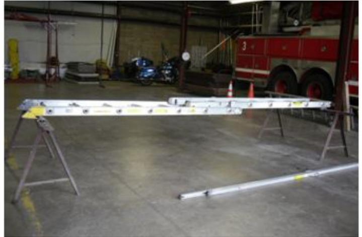
major difference is the weights that will be used. Once the ladder is correctly mounted on the saw horses and the board is positioned, 250 pounds of weights is used; the weight is the same for both time periods during this test.
