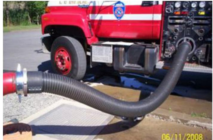
Start the apparatus and engage the pump. Prime the pump by bringing the RPMs up to 1,100. Activate the primer valve and operate the pump as you would during drafting operations. Document the amount of time it took to prime and start flowing water. The acceptable time for a 1,250 GPM pump is 30 seconds or less.
