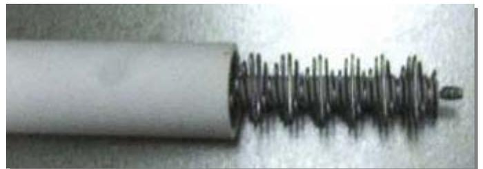
*Fig. 4 – Open coil heater element with insulator tube partially removed.*
