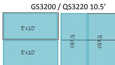
If printer width is less than 3.2 meters wide, a 10' board must be rotated to print short edge first. This increases
