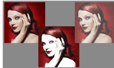
This example shows the 3 files used in the final MaxColor 3-layer print. The simple pre-press technique incorporates 3 layers of color for maximum visual impact. White ink also acts as a diffuser; the pastel appearance of the last layer is a result of CMYK and 100% white ink printing simultaneously.
