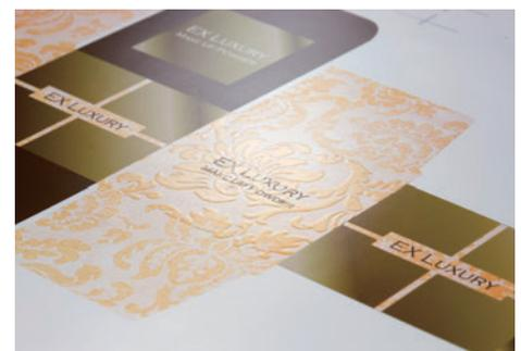
Finishing also includes die-cutting and scoring of the materials. A UV-LED printer featuring integrated contour cutting, such as Roland's LEC-330 and LEC-540, not only prints but also performs scoring, kiss cutting and die cutting
