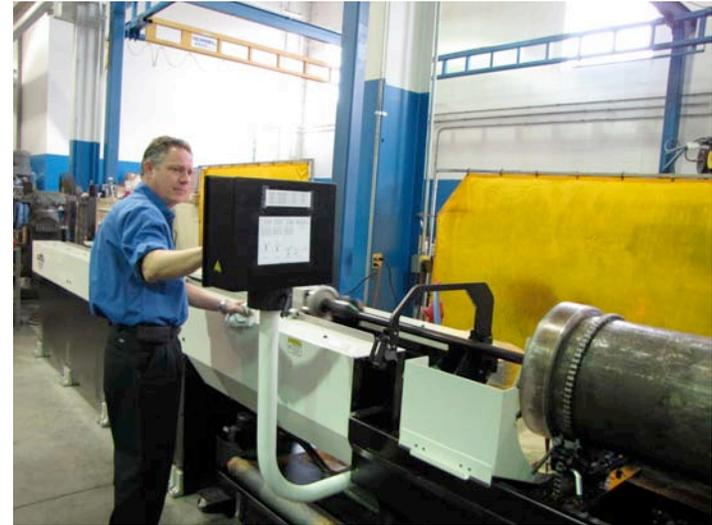
**AirHydro3.jpg:** A touch-screen controlled hone provides a safer working environment and reduces operator fatigue, as well as providing better quality parts by producing a controlled crosshatch pattern, which allows the honed surface to retain oil or grease and ensure proper lubrication.
