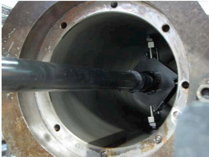
**AirHydro2.jpg:** Transition to the HTA was easy for Air Hydro Power: the machine uses the same Sunnen ANR tooling the shop was using to hand hone.
