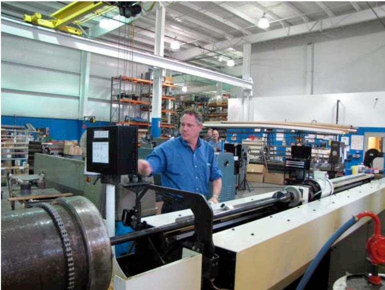
**AirHydro5.jpg:** Air Hydro's Perry Goldstein sets up a Sunnen HTA tube hone to recondition a hydraulic cylinder. The HTA includes a Siemens drive and PLC control with touch-screen HMI for setting machine parameters such as stroke reversal point, spindle/stroking speed and crosshatch angle calculation.
