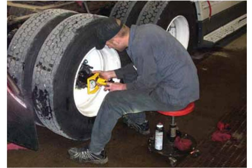
Temper has developed a technology to directly preload the bearings rather than having to torque a locking nut, allowing “measurement” of preload during the adjustment process and fine tuning the bearing set to the optimal preload setting.
